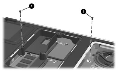
Removing the Keyboard Screws
